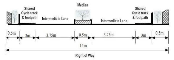
Figure 9: Typical Cross-section for Class A Roads (with RoW 15 m)
