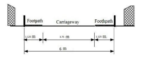
Figure 12: Typical Cross-section for Class D Roads (with RoW 6 m)
