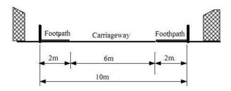
Figure 10: Typical Cross-section for Class B Roads (with RoW 10 m)
