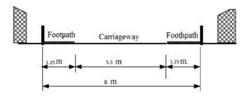
Figure 11: Typical Cross-section for Class C Roads (with RoW 8 m)
